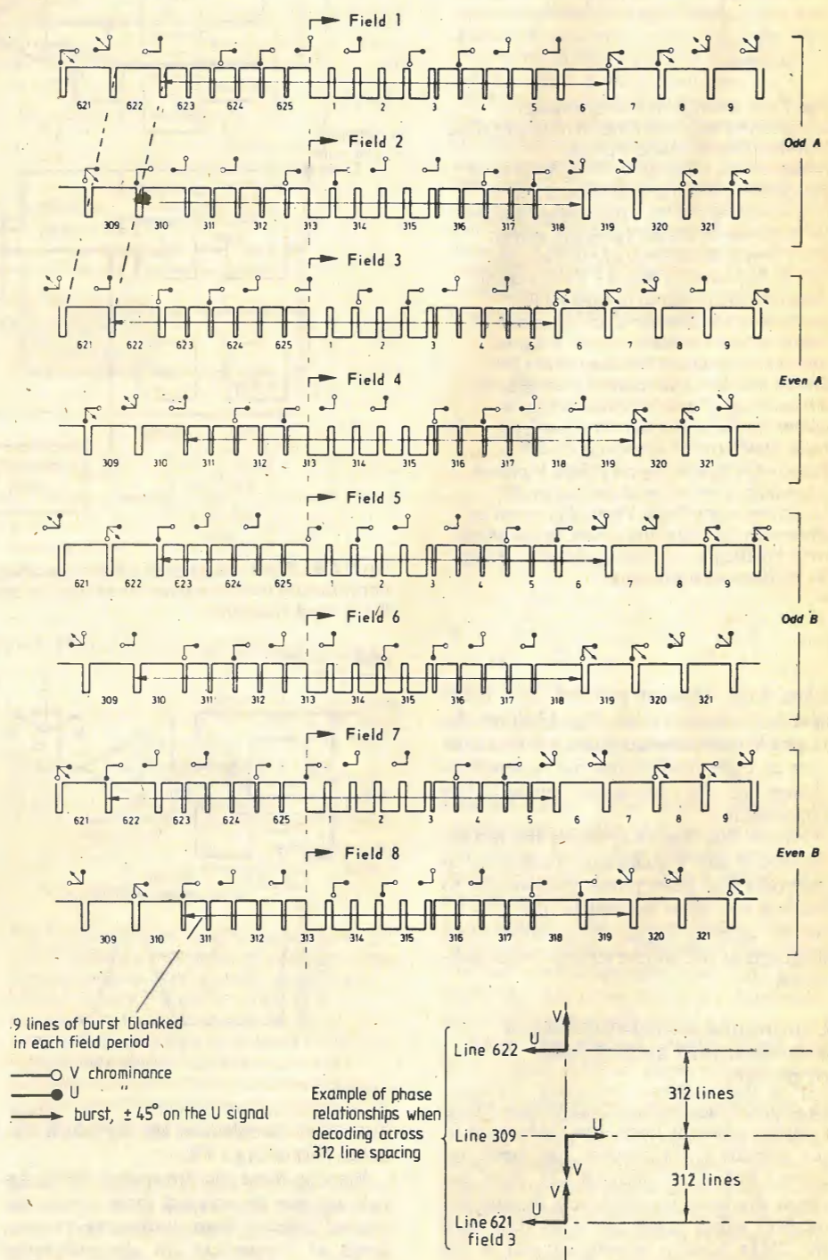
Fig. 13(a). Full eight-field sequence over which the colour subcarrier phase sequence repeats. The pairs of rounded vectors show U/V phases across field and picture intervals. (From EBU statement D22-1979).
